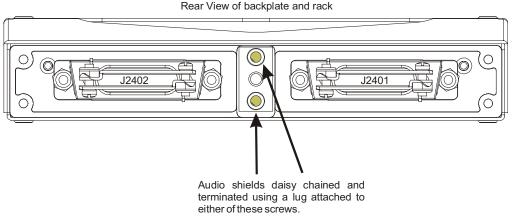
Figure 3-1. Audio Shield Termination
